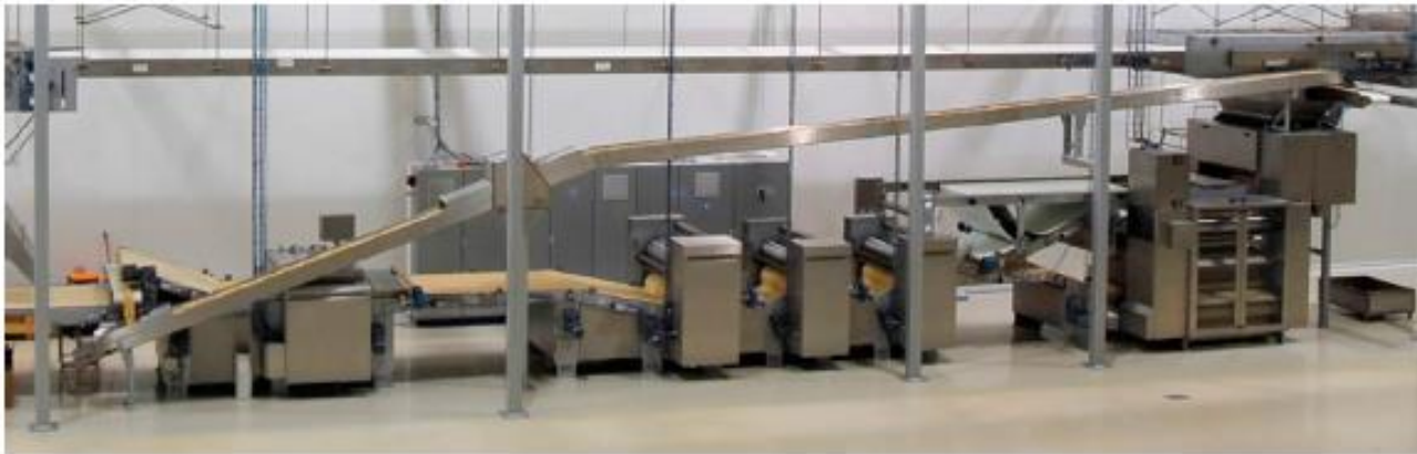
Figure 1.5 Baker Perkins forming line: (right to left) laminator, three gauge roll units, relaxation conveyor, rotary cutter, scrap lift and return conveyors.
